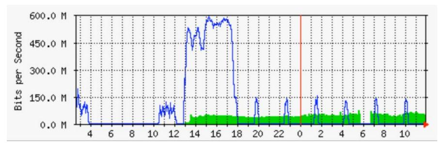
The inbound and outbound network traffic at the NRC cluster in Ottawa. The VMs were stored at NRC and the data at UVIC. The outbound traffic (shown by the blue line) shows the transfer of the 60 VMs to UVIC.
