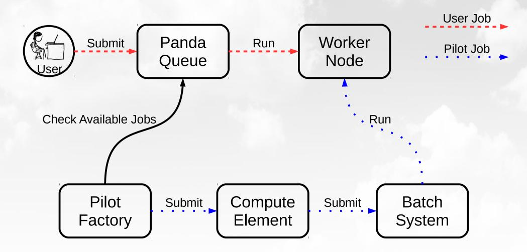
Compute Element is tightly coupled to batch system
